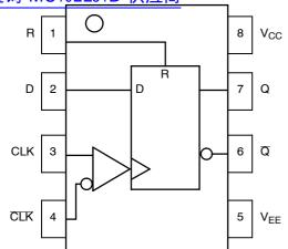
Figure 1. Logic Diagram and Pinout Assignment
