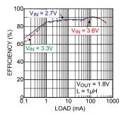
The Figure above shows an efficiency curve. From no load to 100mA, efficiency losses are dominated by quiescent current losses, gate drive and transition losses. By using the Hyper Light Load<sup>TM</sup> mode the MIC23050 is able to maintain high efficiency at low output currents.
