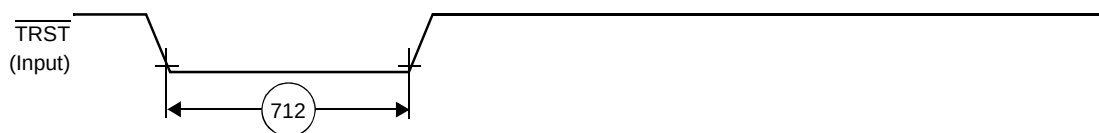
Figure 29. TRST Timing Diagram
