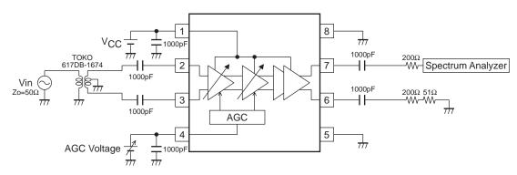
Output Voltage is divided by  $50\Omega$  / (200+50) $\Omega$
