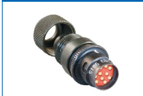
VG96934D10*L0 10 pin in-line unshrouded receptacle with two piece shielded aluminum backshell. 6 mm cable entry. Black zinc plating. Not for new design. Replaced by Style K. Maximum weight 15 grams.
