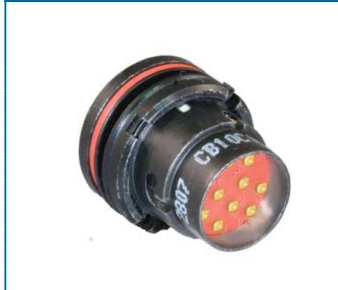
VG96934C10*L* 10 pin jam nut receptacle for rear panel mounting. Maximum weight 11 grams. Stainless steel shell with black chromate.
