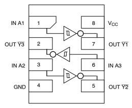
Figure 1. Pinout (Top View)
