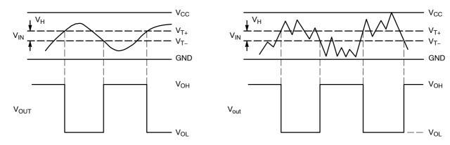
(a) A Schmitt-Trigger Squares Up Inputs With Slow Rise and Fall Times
