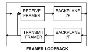
This loopback is useful in testing and debugging applications. In FLB, the DS26556 loops data from the transmit side back to the receive side. When FLB is enabled, the following occurs:
