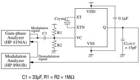
VC modulation signal: 100Hz to 100kHz, 0 to  $V_{DD}$ p-p
