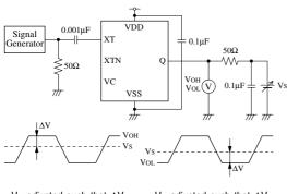
$V_{S}$  adjusted such that  $\Delta V$  = 50  $\times$  I\_{OH}.
