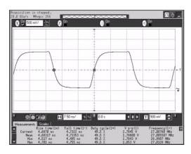
$$\label{eq:VDD} \begin{split} V_{DD} = 1.8 \text{V}, \ \text{f}_{OUT} = 27 \text{MHz}, \ \text{V}_{C} = 0.5 \text{V}_{DD}, \\ C_{LOUT} = 15 \text{pF}, \ \text{Ta} = \text{R.T}. \end{split}$$
