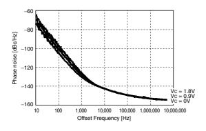
$V_{DD}$  = 1.8V,  $f_{OUT}$  = 27MHz, Ta = R.T.
