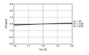
$f_{OUT}$  = 27MHz,  $\pm$  0ppm at  $V_{DD}$  = 1.8V
