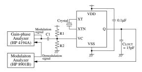
C1 = 33µF, R1 = R2 = 1M $\Omega$  VC modulation signal: 100Hz to 100kHz, 0 to V\_DDP-p
