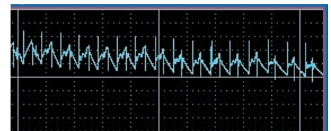
Actual measurement example for inverter current using the 8855 in combination with the 3274
