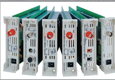
FUNCTION UP DISK 9549 Power monitor function add in to the MEMORY HiCORDER 8855
