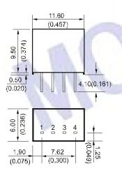
Note: Unit:mm(inch) Pin section:0.50\*0.30mm(0.020\*0.012inch) Pin tolerances:±0.10mm(±0.004inch) General tolerances:±0.25mm(±0.010inch)
