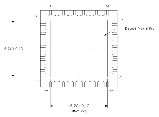
NOTE: All linear dimensions are in millimeters
