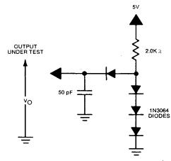
Capacitive loading to simulate effect of five additional outputs plus one TTL input
