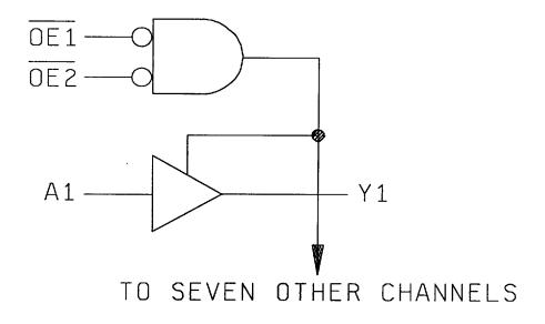
FIGURE 3. Logic diagram.
