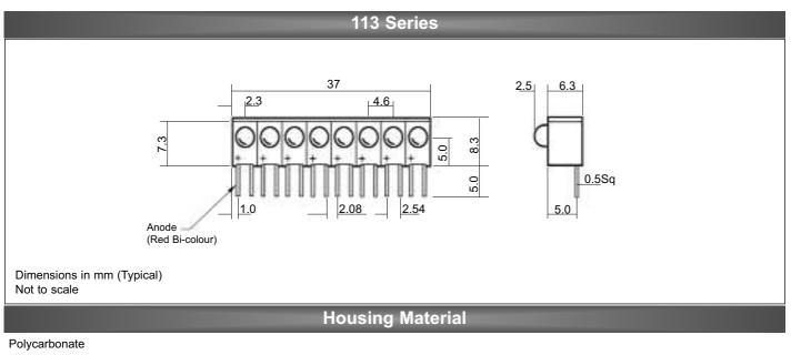
This material offers UL94 V-0 flame retardancy\* and a high impact strength. This material has a melt point of 290-340°C and is suitable for use in the majority of automatic soldering processes.
