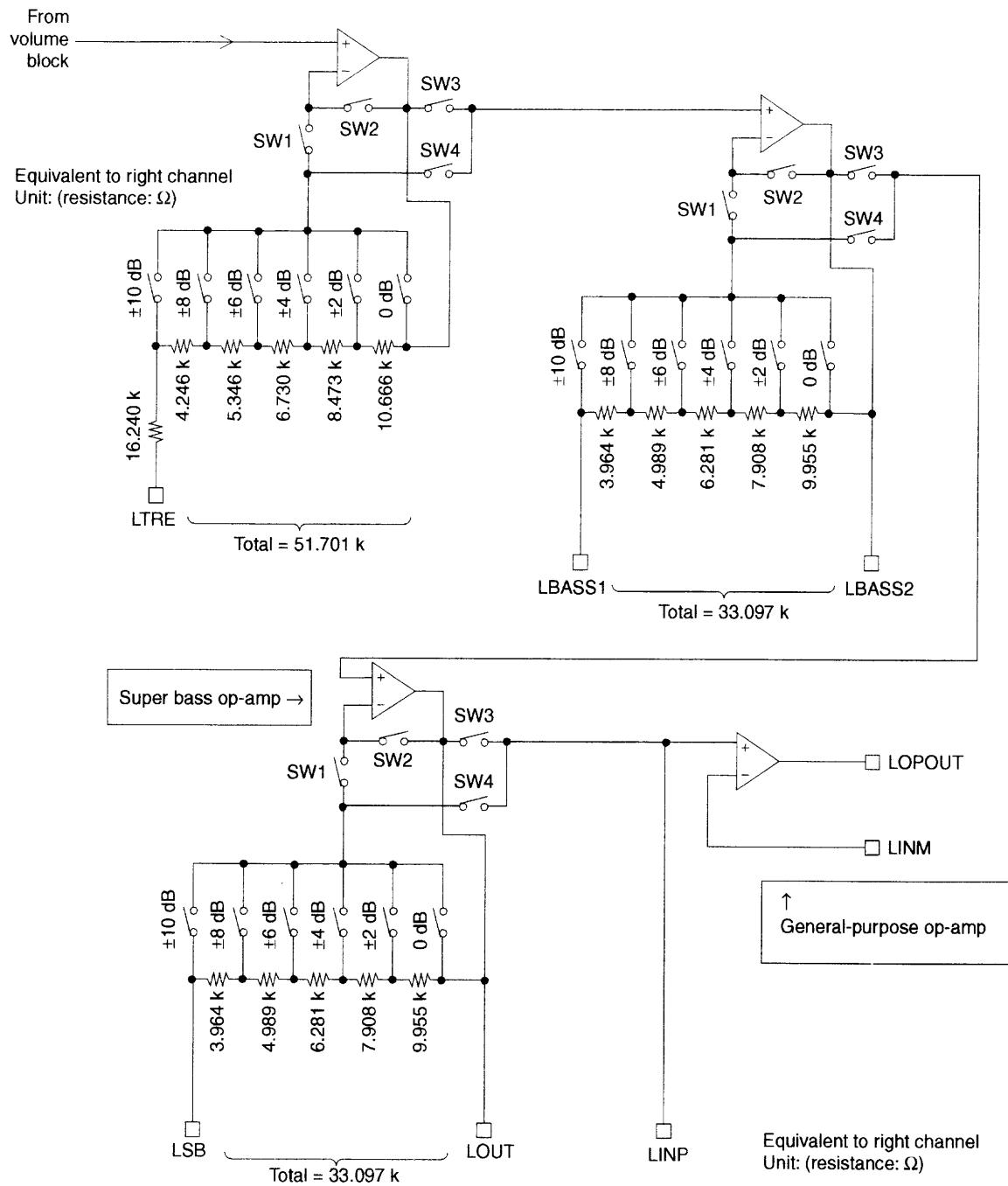
During boost, SW1 and SW3 are on, during cut, SW2 and SW4 are on, when 0 dB, 0dB SW and SW2 and SW3 are on.
