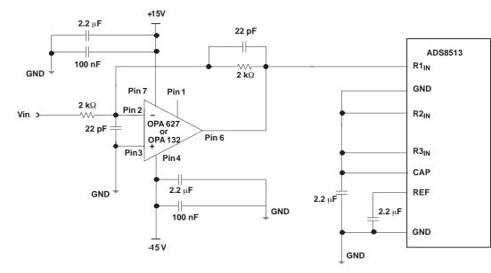
Figure 11. Typical Driving Circuit (±10 V, No Trim)
