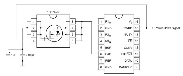
Figure 14. Improved Power-Up Response Circuit
