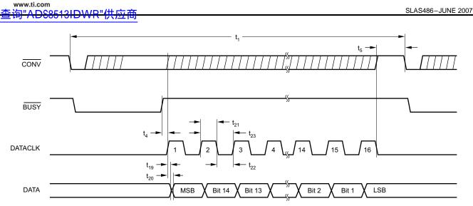
Figure 7. Serial Data Timing, External Clock, Clocking After the Conversion Completes (EXT/INT High, CS Low)
