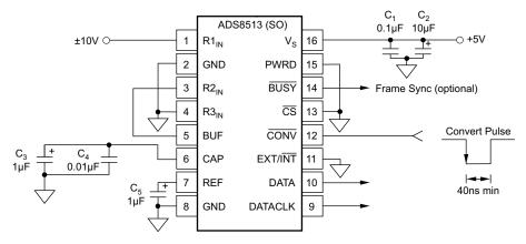
Figure 1. Basis Operation, ±10-V Input Range, Internal DATACLK
