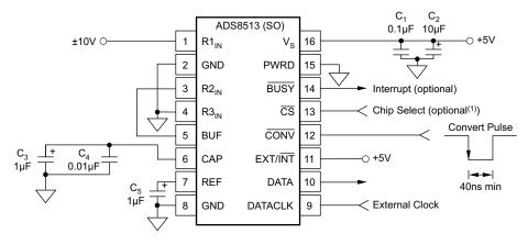
NOTE: (1) Tie  $\overline{CS}$  to GND if the outputs will always be active.
