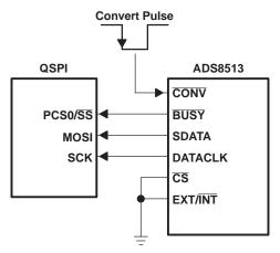
CPOL = 0 (Inactive State is LOW) CPHA = 1 (Data Valid on Falling Edge) QSPI Port is in Slave Mode.
