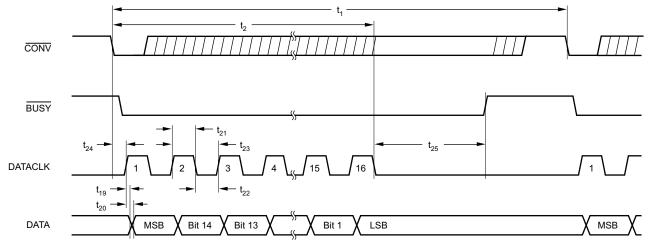
Figure 8. Serial Data Timing, External Clock, Clocking During the Next Conversion (EXT/INT High, CS Low)
