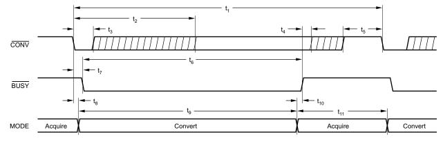
Figure 3. Basic Conversion Timing
