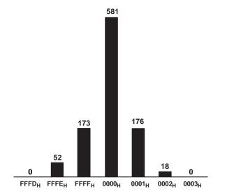
Figure 16. Histogram of 1000 Conversions With Input Grounded
