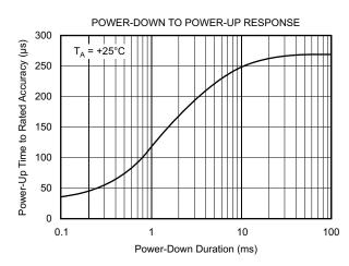
Figure 13. Power-Down to Power-Up Response
