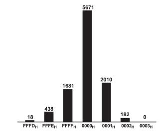
Figure 17. Histogram of 10000 Conversions With Input Grounded
