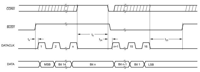
Figure 9. Serial Data Timing, External Clock, Clocking <u>After the Conversion</u> Completes and During the Next Conversion (EXT/INT High, CS Low)
