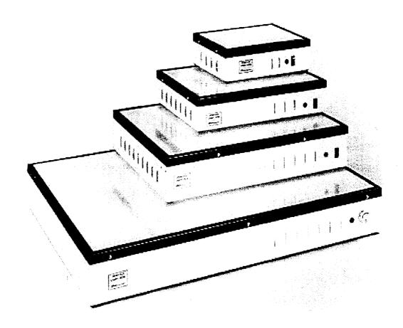
High quality light boxes - an invaluable aid to any artwork preparation. Each case is constructed from 18 gauge steel featuring air vents in four sides and is completed using sheets of 050 opal perspex and glass which is secured by a black lid surround. This ensures both even temperature and illumination. The glass top means that a scalpel may be used to trim artworks directly on the illuminated surface.
