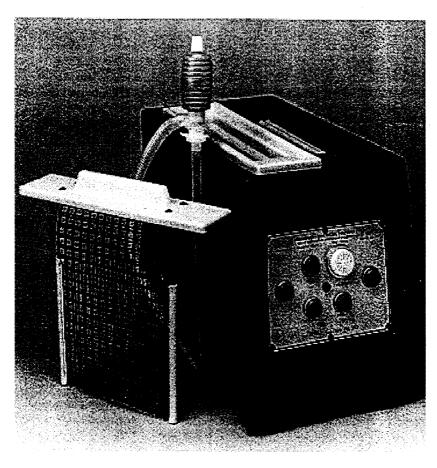
An improvement standard over а Bubble Etch Tank This unit is the same as the PA104 Bubble Etch Tank with the addition of an integral spray wash tank. The spray wash is solenoid operated and all electrical controls are on the front panel. Connections are provided at the rear for drain and cold water requirements. The integral spray offers wash tank safer and more
