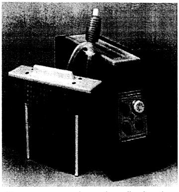
This, the most popular of single tanks, includes the heater and thermostat sensor as described above and has a pump fitted which forces air through two bubble bars to provide efficient and even etching. Supplied illuminated switches control mains power and the pump whilst a neon indicates heater operation. The switches and neon have splash proof covers.
