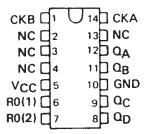
SN5493A, SN54LS93 . . . J OR W PACKAGE SN7493 . . . N PACKAGE SN74LS93 . . . D OR N PACKAGE (TOP VIEW)
