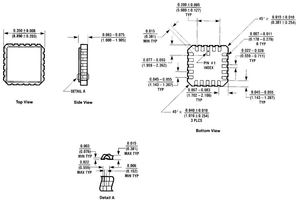
20-Lead Ceramic Leadless Chip Carrier (L)
