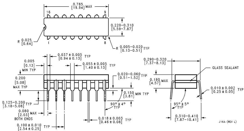
16-Lead Ceramic Dual-In-Line Package (D)
