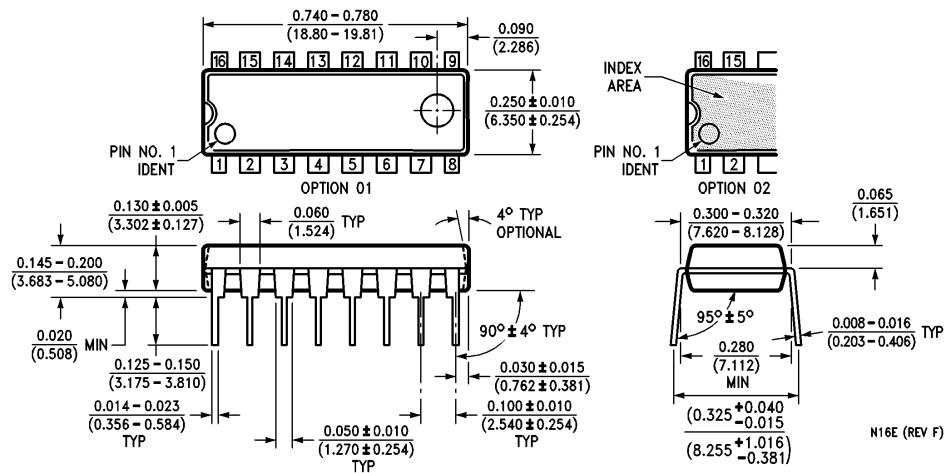
16-Lead (0.300" Wide) Molded Dual-In-Line Package (P)
