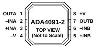
Figure 1. 8-Lead, Narrow-Body SOIC (R-8)
