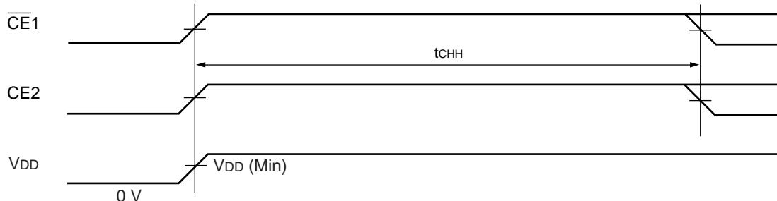
Note :  $t_{CHH}$  specifies after  $V_{DD}$  reaches specified minimum level and applicable to both  $\overline{CE1}$  and  $CE2$ .
