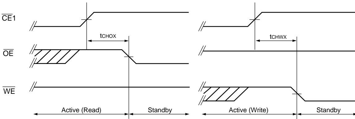
Note : Both  $t_{CHOX}$  and  $t_{CHWX}$  define the earliest entry timing for Standby mode.
