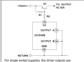
grounded. The VC terminal is switched to ground by the totem-pole source transistors on alternate oscillator cycles.
