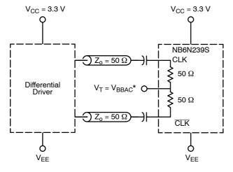
Figure 16. Capacitor–Coupled Differential Interface (V<sub>T</sub> Connected to V<sub>BBAC</sub>)
