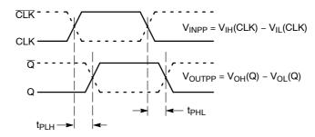
Figure 19. AC Reference Measurement
