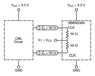
Figure 14. Standard 50  $\Omega$  Load CML Interface
