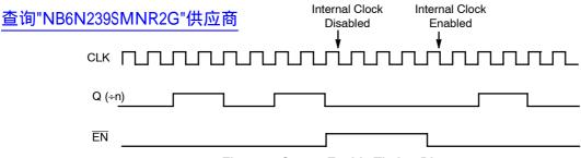
Figure 6. Output Enable Timing Diagrams
