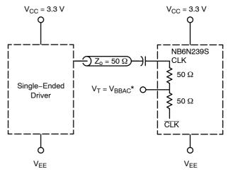
Figure 17. Capacitor–Coupled Single–Ended Interface ( $V_T$  Connected to  $V_{BBAC}$ )
