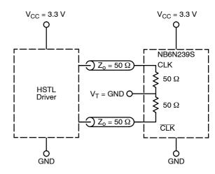
Figure 15. Standard 50  $\Omega$  Load HSTL Interface
