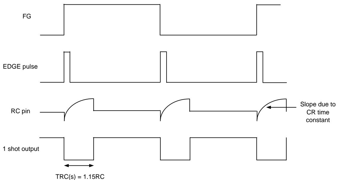
Furthermore, by changing the pulse width as determined by the CR time constant, the VCTL versus speed slope can be changed as shown in the speed control diagram of the previous section.
