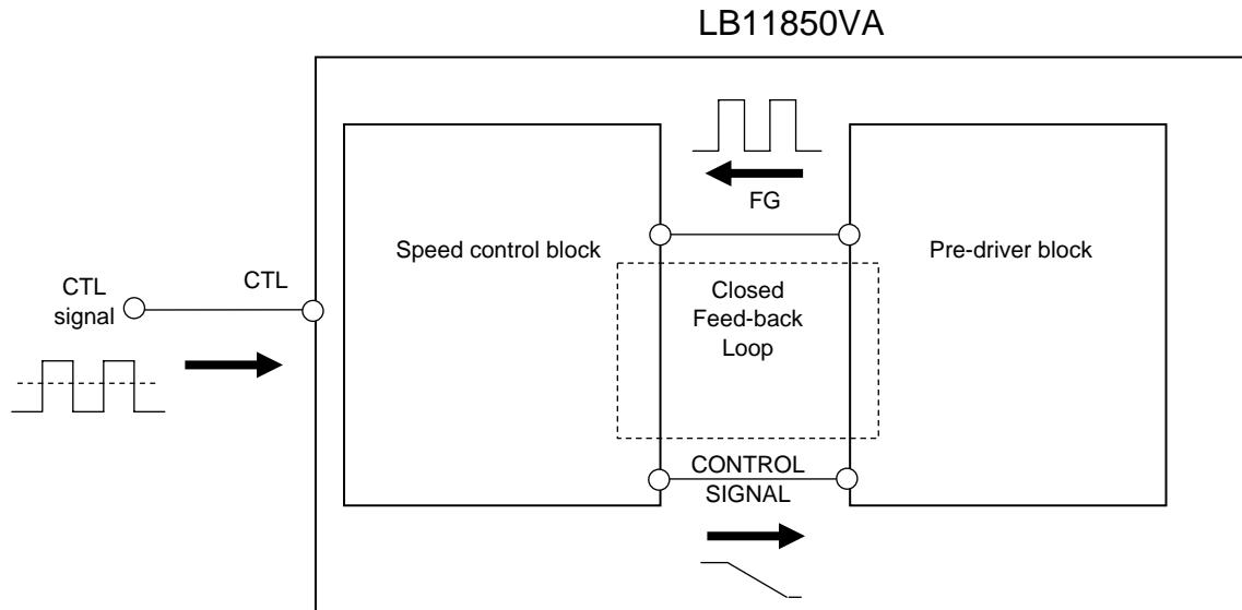
The operation inside the IC is as follows. Pulse signals are created from the edges of the FG signals as shown in the figure below, and a waveform with a pulse width which is determined by the CR time constants and which uses these edges as a reference is generated by a one-shot multivibrator.
