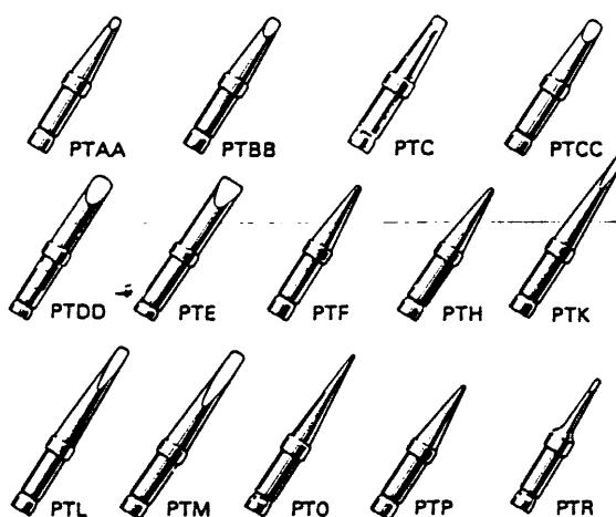
"Longlife" tips are made from pure copper, then iron plated for long life and chromium plated to prevent oxidation. With proper care they are always wettable.
