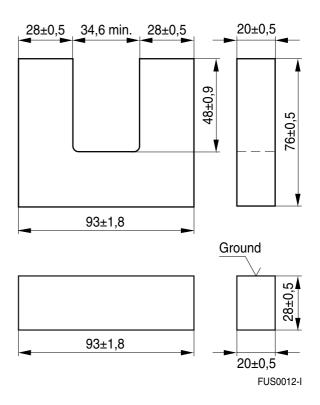
U and I cores are supplied as single units. The  $A_{\rm L}$  value in the table applies to a core set comprising two ungapped cores.
