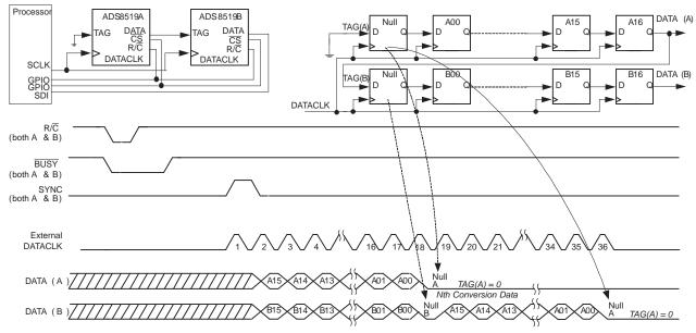
EXT/INT tied high, CS of both converter A and B, TAG input of converter A are tied low.
