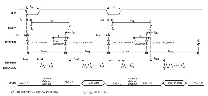
Figure 3. Basic Conversion Timing: External DATACLK
