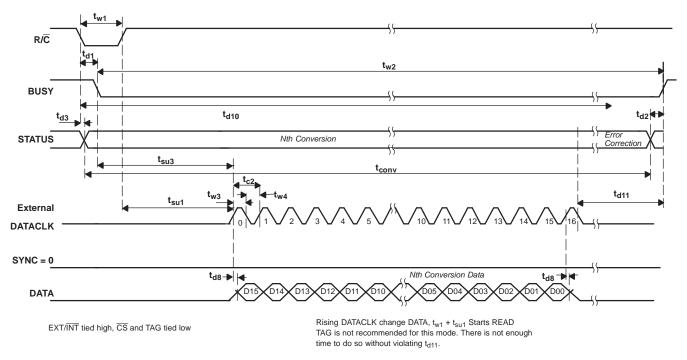
Figure 5. Read During Conversion (Discontinuous External DATACLK)
