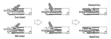
Alternating even spring terminals and odd stationary terminals provide opposing forces for high FPC retention force.
