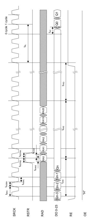
$t_{RAE}$  (=21clk): Period of Address input from Read Reset. After read reset, RE should be remained high for 2 cycles after driving RE high first.
