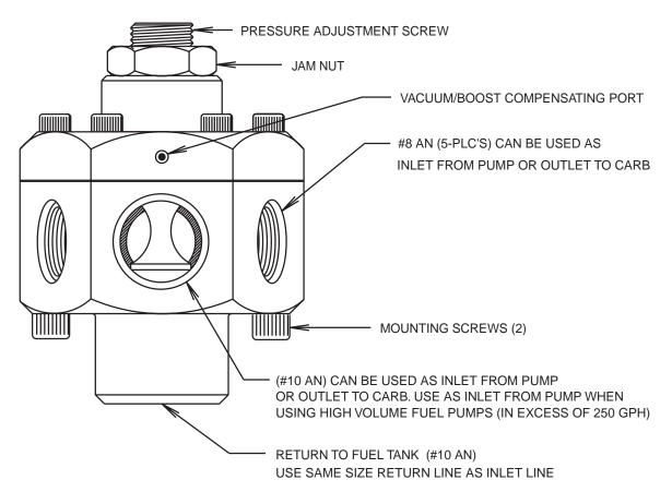
NOTE: A bypass at the fuel pump is not required for this regulator. When using this regulator with Mallory Series 5250 or 5500 fuel pumps, the fuel return port at the pump should be plugged.
