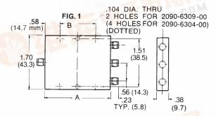
Note: All dimensions are ±.020, except mounting hole diameters (±.005) and mounting hole location (±.010). Height dimension excludes rivet protrusion.
