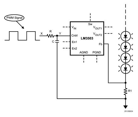
FIGURE 3. If V<sub>OUT2</sub> is not used, En2 must be grounded
