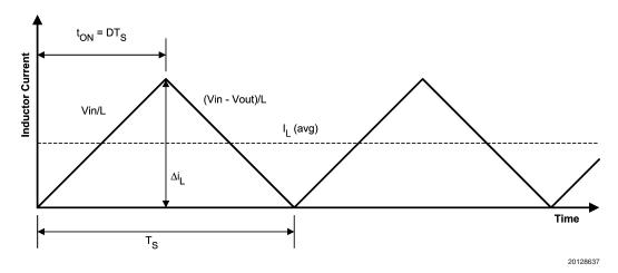
FIGURE 4. Inductor Current Waveform
