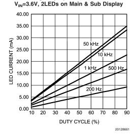
**Dimming Duty Cycle vs. LED Current**
