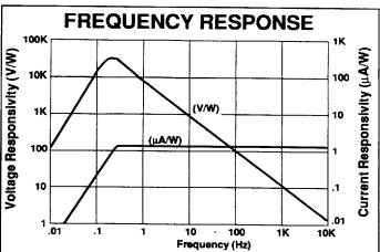
The current response of the Model 400 to modulated radiant energy (pulsed or chopped) is flat beyond the thermal break and is shown on the designated curve with appropriate dimensioning on the right ordinate axis. Response of the Model 400 through a source follower (ELTEC Model 320 set at 5x10<sup>10</sup>) is shown on the left ordinate axis.
