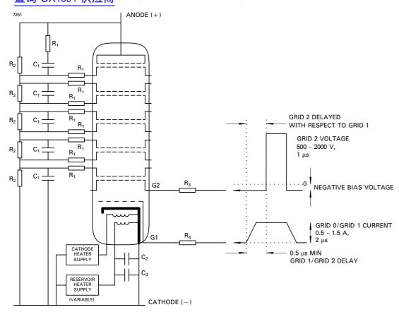
$R_1 = 470 \Omega 12 W$  vitreous enamelled wirewound resistors.
