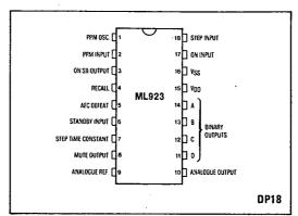
Fig.1 Pin connections (top view)
