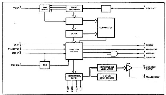
Fig.2 ML923 block diagram
