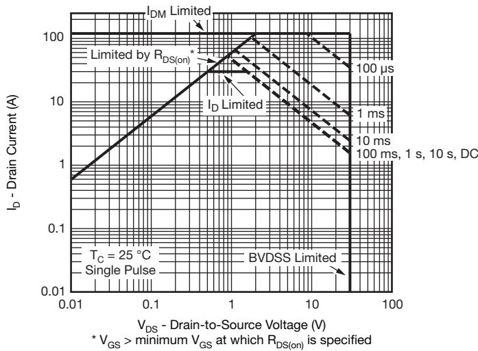
**Safe Operating Area**
