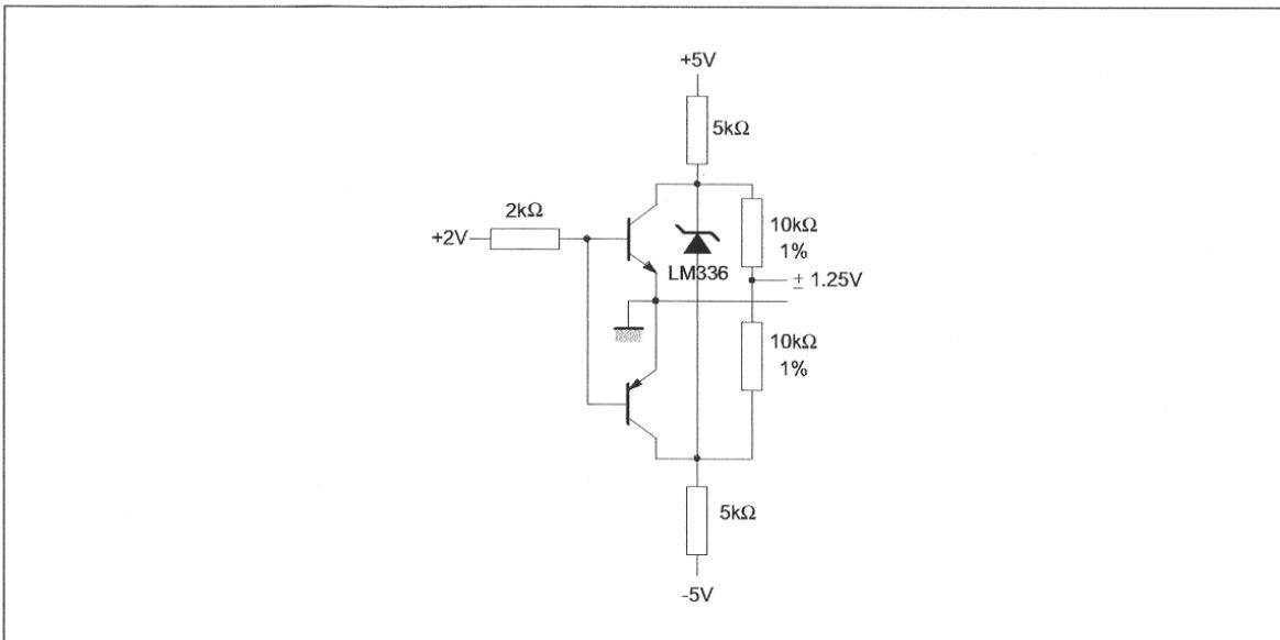
Figure 9 : 5V Buffered Reference
