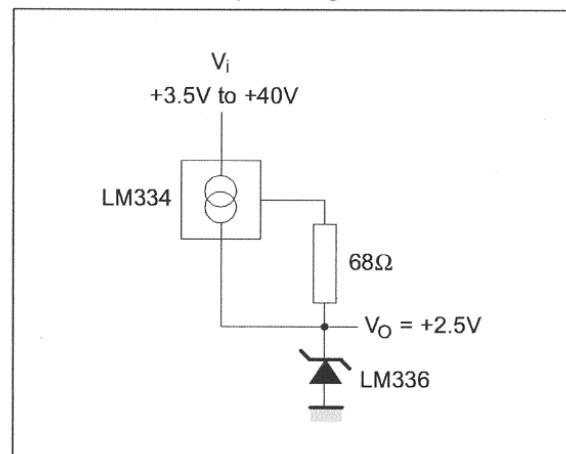
Figure 5 : Precision Power Regulator with Low Temperature Coefficient
