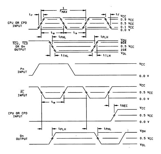
FIGURE 4. Switching waveforms and test circuit.
