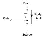
**Remark** Strong electric field, when exposed to this device, can cause destruction of the gate oxide and ultimately degrade the device operation. Steps must be taken to stop generation of static electricity as much as possible, and quickly dissipate it once, when it has occurred.
