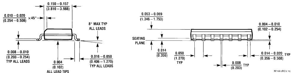
14-Lead Small Outline Integrated Circuit (SOIC), JEDEC MS-120A, 0.150" Narrow Package Number M14A
