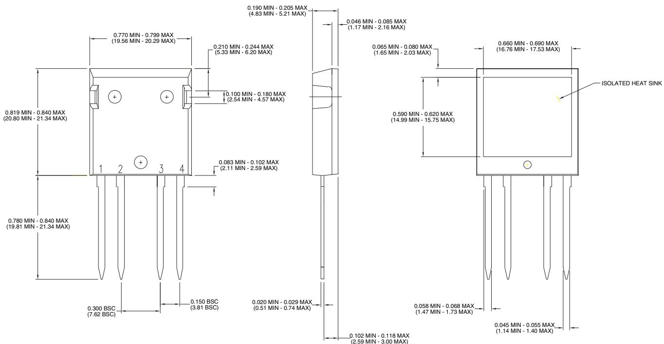
NOTE: Bottom heatsink meets 2500V<sub>rms</sub> isolation to the other pins.
