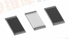
These chip resistors are available in wraparound terminations styles in 8 case sizes. They incorporate self passivated enhanced tantalum nitride resistor film to give superior performance on moisture resistance, electrostatic discharge, voltage coefficient, power handling and resistance stability. The terminations consist of an adhesion layer, a leach resistant nickel barrier, and solder coating (lead (Pb)-free). This product will out-perform all requirements of AEC-Q200.
