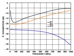
Figure 9. S11, S12 and S22 Vs. Frequency
