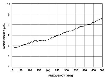
Figure 8. Noise Figure Vs. Frequency at Max Gain
