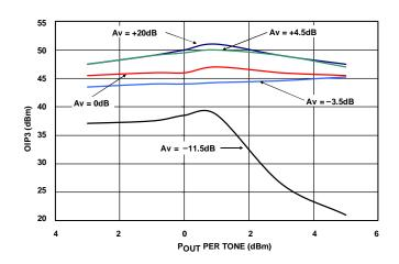
Figure 5. OIP3 vs. Power @ 5 Gains
