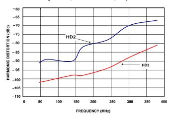
Figure 10. Harmonic Distortion Vs. Frequency 2Vp-p Out
