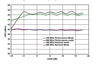
Figure 7. OIP3 Vs. Gain
