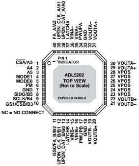
Figure 2. 40 Lead LFCSP
