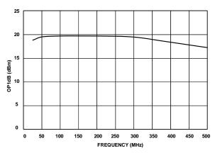
Figure 6. P1dB Vs. Frequency at Max Gain
