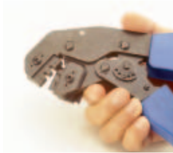
2. While pressing upward on the locator spring, insert the contact with tails upward completely into the locator.
