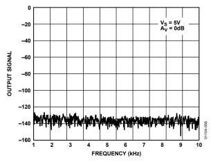
Figure 56. Spectral Analysis of AD8572 Output in Unity Gain Configuration
