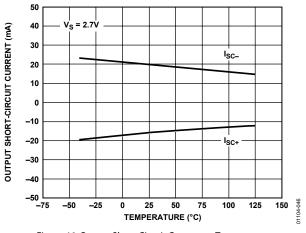
Figure 46. Output Short-Circuit Current vs. Temperature
