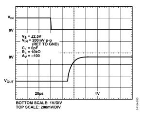
Figure 30. Negative Overvoltage Recovery
