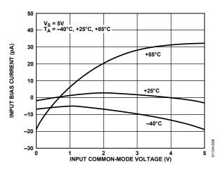
Figure 8. Input Bias Current vs. Input Common-Mode Voltage
