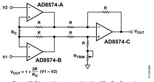
Figure 65. Discrete Instrumentation Amplifier Configuration
