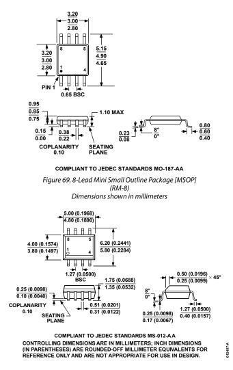
Figure 70. 8-Lead Standard Small Outline Package [SOIC\_N] Narrow Body (R-8) Dimensions shown in millimeters and inches
