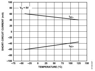
Figure 47. Output Short-Circuit Current vs. Temperature
