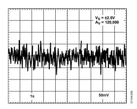
Figure 39. 0.1 Hz to 10 Hz Noise at 5 V
