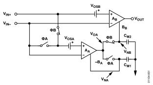
Figure 51. Output Phase of the Amplifier
