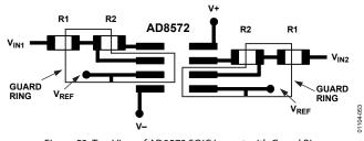
Figure 53. Top View of AD8572 SOIC Layout with Guard Rings
