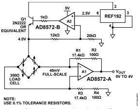
Figure 63. 5 V Precision Strain Gage Amplifier
