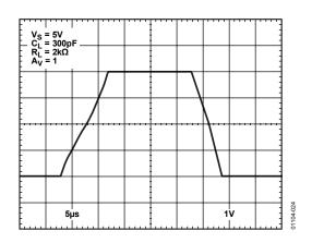
Figure 24. Large Signal Transient Response at 5 V
