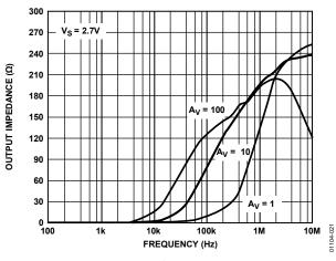
Figure 21. Output Impedance vs. Frequency at 2.7 V
