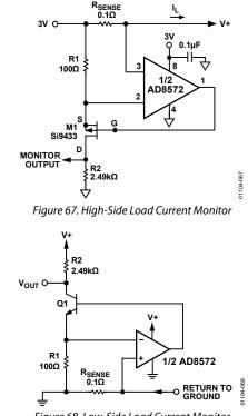
Figure 68. Low-Side Load Current Monitor
