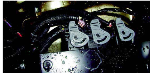
CMC Connectors in Engine Application
