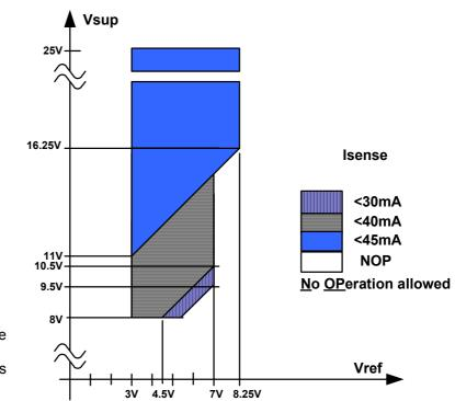
The operating range, and the corresponding maximum Isense, is defined by the Vsup-Vref range as shown in the graph.
