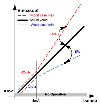
In the above graph the errors values are shown in Current Mode. Down to 5mA %Meas\_lerr1 and below 5mA IMeas\_lerr2.
