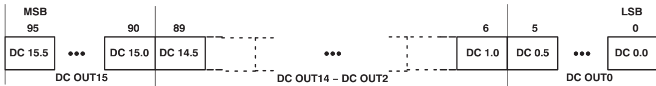
Figure 15. Dot Correction Data Packet Format
