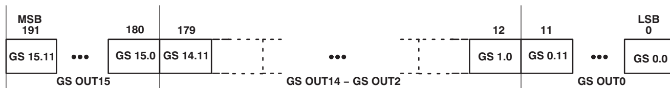
Figure 19. Grayscale Data Packet Format
