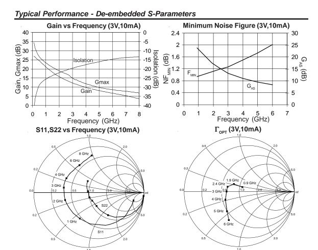
Note: S-parameters are de-embedded to the device leads with  $Z_s = Z_L = 50\Omega$ . The device was mounted on a 0.010" PCB with plated-thru holes close to pins 2 and 4. De-embedded s-parameters can be downloaded from our website (www.sirenza.com).
