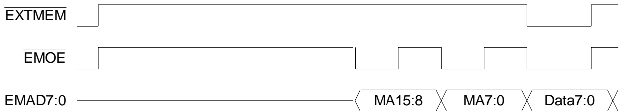
Figure 22. Run-Time Memory Access
